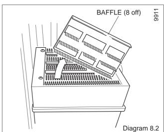
Clean the heat exchanger flueways with a suitable stiff brush. Remove the paper together with any debris.
